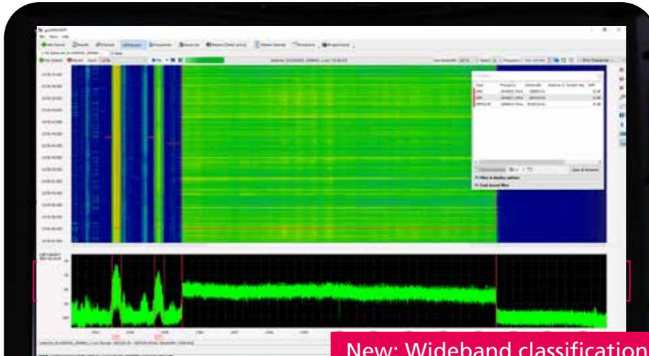
New: Wideband classification of UMTS/LTE emissions (example LTE signal with 10 MHz)
